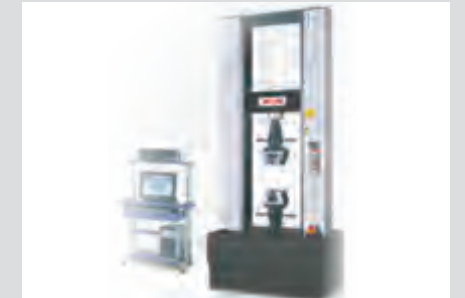
UTM5105X型微机控制电子万能试验机 UTM5105X Floor-Standing Electromechanical Universal Testing Machine
