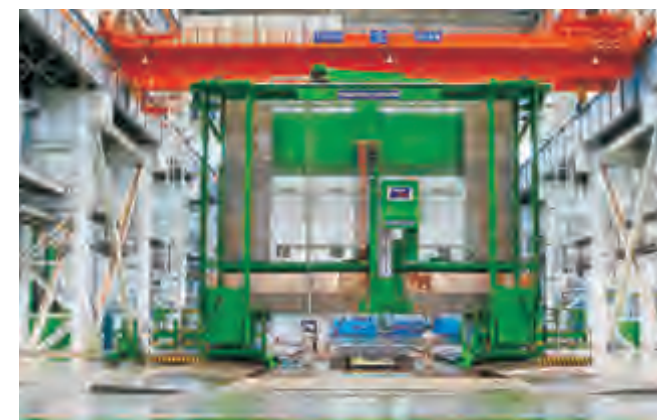
52.5米x8米x8米 数控龙门镗铣床 52.5mx8mx8m Digital Control Gantry Boring & Milling Machine
