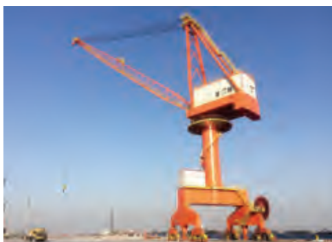
40t x 85m 门座起重机 40t x 85m Portal Crane
