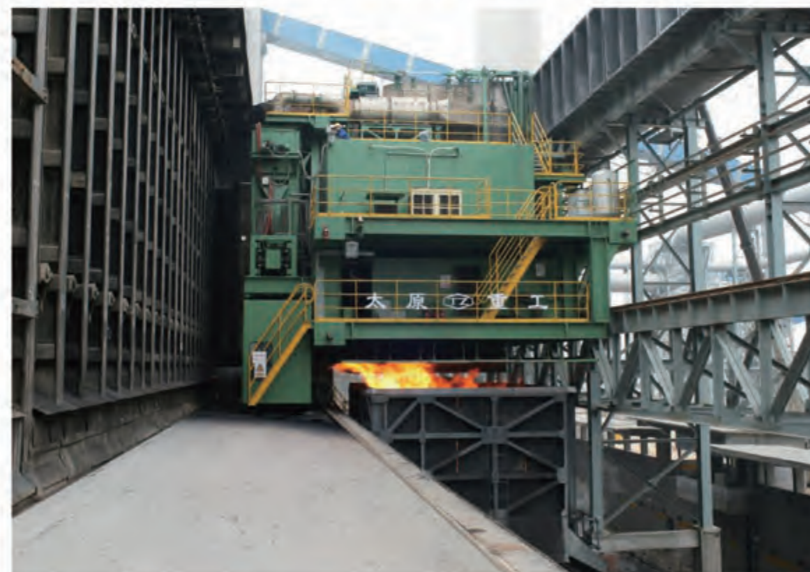
7.3m顶装焦炉推焦车技术参数 Top-charging Coke Oven Machinery (Parameters of 7.3m)
