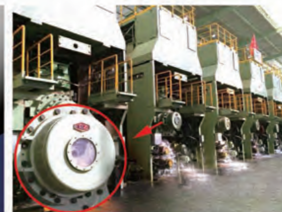
板带轧机油膜轴承 Oil Film Bearing for Strip Mill
