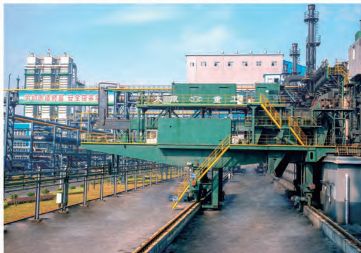
6.78m捣固焦炉装煤车技术参数 Tamping Coke Oven Machinery (Parameters of 6.78m)
